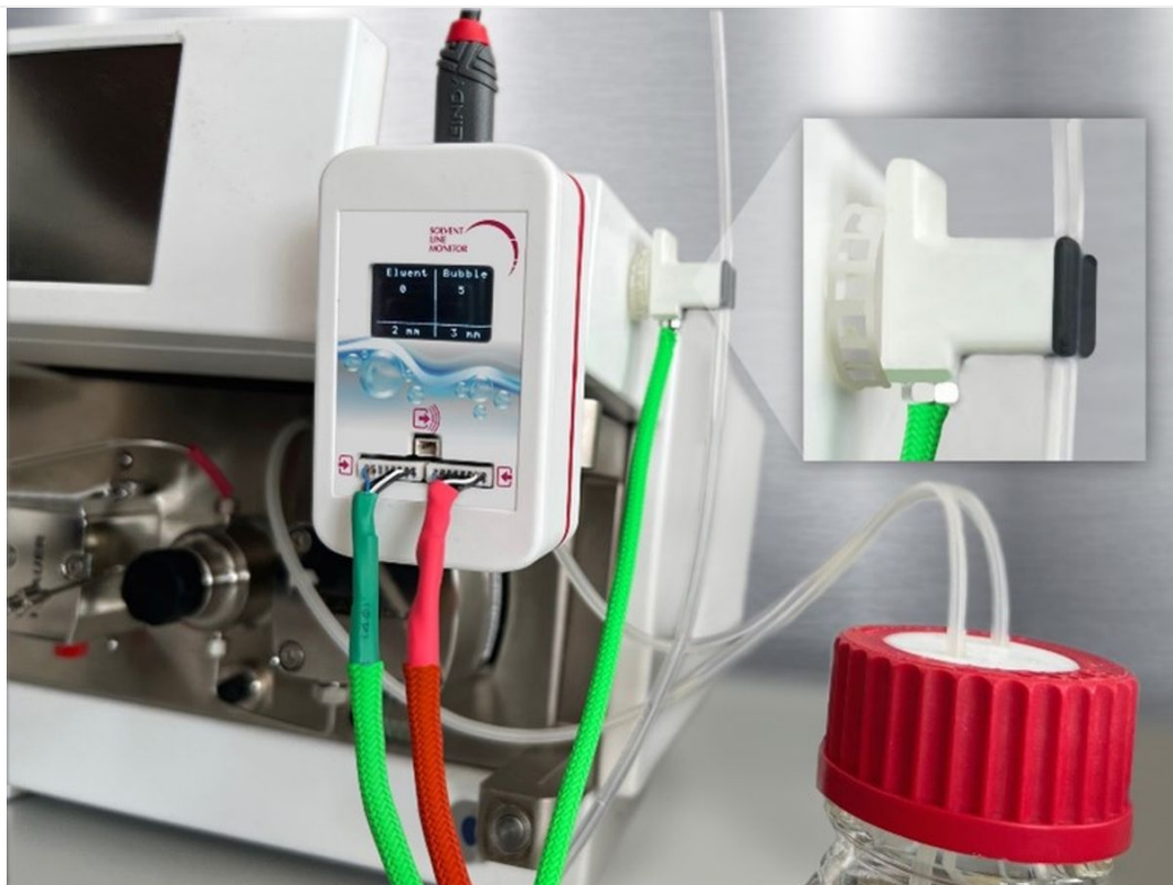
Figure 5: A mechanism to alert for undissolved gas bubbles
