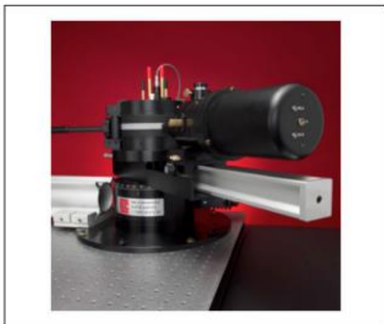
Figure 1: A goniometer based light scattering instrument.
