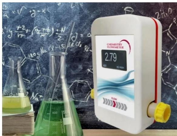
**Carlo Dessy:** As our flow sensor does not interfere with the measurement it can operate over a wide dynamic range. It has been demonstrated to be the perfect real-time flow monitoring tool for liquid chromatography applications including calibrating the flow rate of HPLC and GPC/SEC pumps, troubleshooting defective systems, and offering continuous validation of products operating in a regulated environment.
